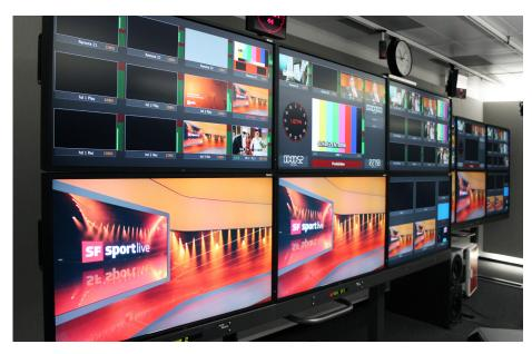
decision was clear-cut and today twentyfour 46inch P461 and seventeen 40inch P401 provide reliable services in the studios. These are fitted out with HD-SDI boards and can also be comfortably operated using the Remote Control Kit.
